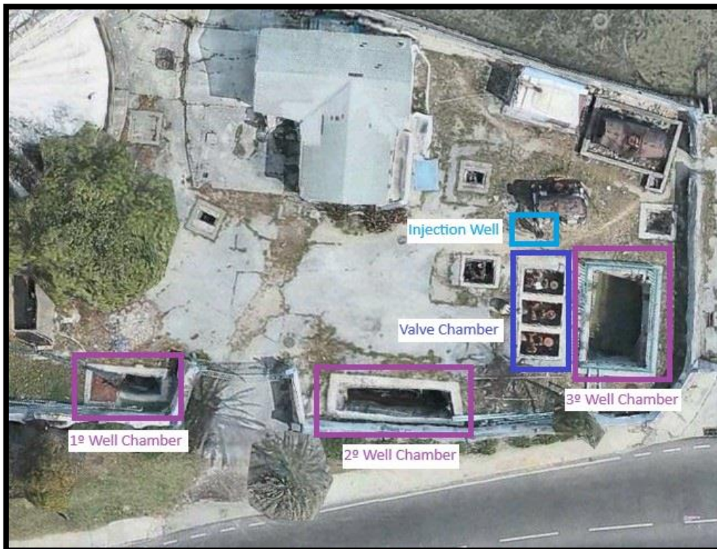
Figure 30. Malcom Lift Station Layout. Source: PlanEHS, 2024.
